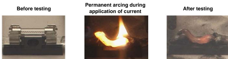
【Figure 2】 Example of a breaking test where the circuit voltage is higher than the rated voltage of the fuse
