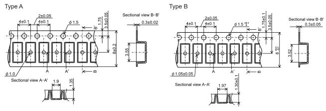
After November 1, 2024, the carrier tape Type A will be switched over to Type B, upon running out of stock of Type A.
