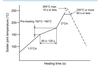
Soldering can be repeated two times under the conditions above.
