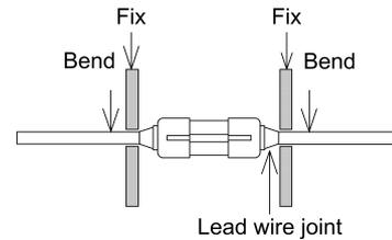
When you form the lead wire, do not apply any excessive stress to the lead wire joint by securely fixing the position between the fuse body and the part subjected to forming as shown in the figures.
