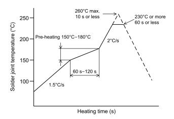
Soldering can be repeated two times under the conditions above.
