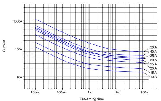
These I-t curve plots are of the average values of the measurements obtained under the conditions specified by our company.
