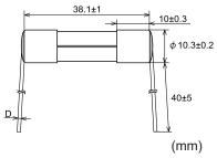
Rated current D 500 mA-8 A:  $\phi$  0.8 Over 8 A-15 A:  $\phi$  1.0 Over 15 A-30 A:  $\phi$  1.2
