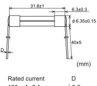
100 mA-8 A: $\phi$  0.8Over 8 A-15 A: $\phi$  1.0Over 15 A-20 A: $\phi$  1.2
