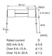
Tube: Lead-free glass End-cap: Nickel plated brass Lead wire: Tin plated copper Solder: 500 mA-12 A Sn-0.7Cu Over 12 A-30 A Pb90-Sn\*1 Adhesive: Epoxy resin Marking: 500 mA-less than 1 A SOC [rated current] 125V 1 A-30 A SOC [rated current] <₽>125V
