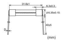
Rated current D 100 mA-8 A:  $\phi 0.8$ Over 8 A-15 A:  $\phi 1.0$ Over 15 A-20 A:  $\phi 1.2$  Tube: Lead-free glass
