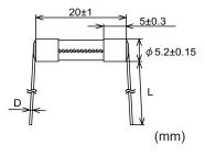
Rated current D L 100 mA-less than 5 A:  $\phi$  0.5 30±5 5 A-10 A:  $\phi$  0.8 40±5
