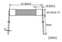
Rated current D 100 mA-8 A:  $\phi 0.8$ Over 8 A-15 A:  $\phi$  1.2
