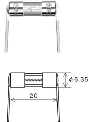
Lead wire diameter  $\phi$  1.2      Scale: 1/1 (mm)
