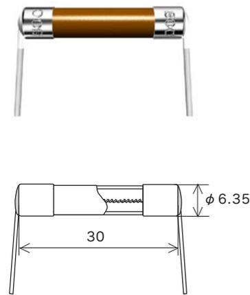
Lead wire diameter  $\phi$  1.2      Scale: 1/1 (mm)
