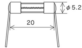
Lead wire diameter  $\phi$  0.5 (100 mA–1 A)  $\phi$  0.8 (Over 1 A–10 A)  $\phi$  1.0 (Over 10 A–15 A) Scale: 1/1 (mm)
