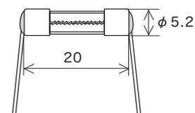
Lead wire diameter  $\phi$  0.5 (100 mA–1 A)  $\phi$  0.8 (Over 1 A–3.5 A) Scale: 1/1 (mm)
