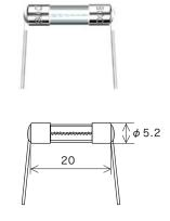
$\begin{array}{ccc} \mbox{Lead wire diameter} & \phi \ 0.8 & (\mbox{Over} \ 3.5 \mbox{ A} - 10 \mbox{ A}) \\ & \phi \ 1.0 & (\mbox{Over} \ 10 \mbox{ A} - 15 \mbox{ A}) \end{array}$
