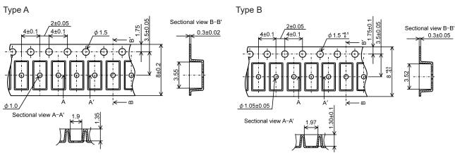
After November 1, 2024, the carrier tape Type A will be switched over to Type B, upon running out of stock of Type A.
