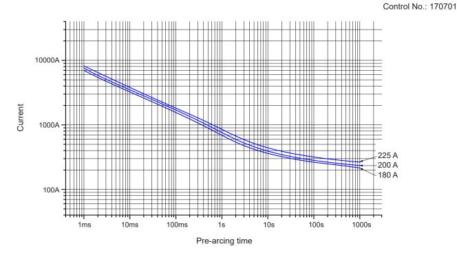
These I-t curve plots are of the average values of the measurements obtained under the conditions specified by our company.
