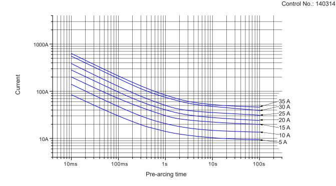
These I-t curve plots are of the average values of the measurements obtained under the conditions specified by our company.
