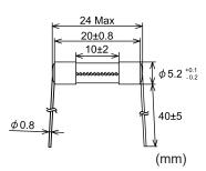
Tube: End-cap: Lead wire: Solder: Adhesive: Marking: Lead-free glass Nickel plated brass Tin plated copper Sn-0.7Cu Epoxy resin T [rated current] E250V ET6R (S) (S) SOC
