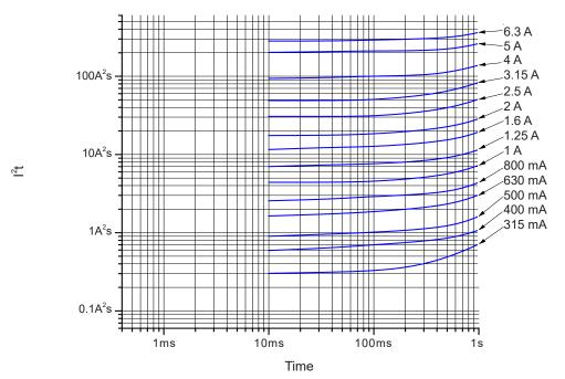
These data are for reference only and are not intended to infer any guaranteed values. Characteristics of the fuse may vary depending on the usage conditions. Always test the fuse under the actual circuit conditions.
