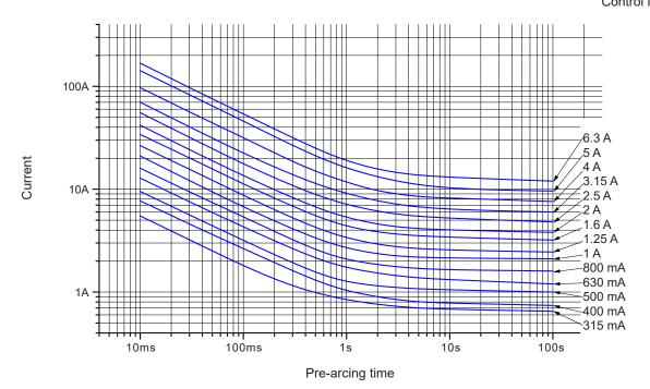
These I-t curve plots are of the average values of the measurements obtained under the conditions specified by our company. Control No.: 050401
