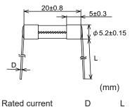
D 100 mA-1 A: φ0.5 30±5 Over 1 A-3.5 A: φ0.8 40±5 Tube: End-cap: Lead wire: Solder: Adhesive: Marking:
