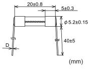
Rated current D Over 3.5 A-10 A:  $\phi$  0.8 Over 10 A-15 A:  $\phi$  1.0 Tube: Lead-free glass
