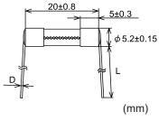
Rated current D 100 mA-1 A:  $\phi$  0.5 30±5 Over 1 A-10 A:  $\phi$  0.8 40±5 Over 10 A-15 A:  $\phi 1.0$ 40±5 Tube: Lead-free glass End-cap: Nickel plated brass Lead wire: Tin plated copper
