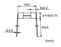
Tube: Lead-free glass End-cap: Nickel plated brass Lead wire: Tin plated copper Solder: Sn-0.7Cu Epoxy resin Adhesive:
