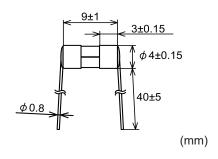
Tube: Lead-free glass End-cap: Nickel plated brass Lead wire: Tin plated copper Pb87.5-Sn10.0-Ag2.5\* Solder:
