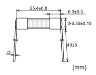
Rated current D 1 A-8 A:  $\phi$  0.8 Over 8 A-less than 15 A:  $\phi$  1.0 15 A-30 A:  $\phi$  1.2
