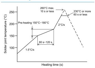
Soldering can be repeated two times under the conditions
