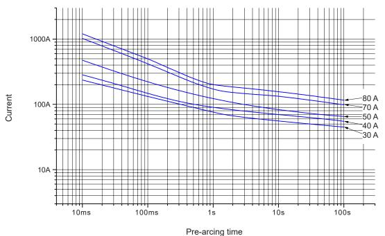
These I-t curve plots are of the average values of the measurements obtained under the conditions specified by our company.
