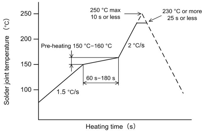
Soldering can be repeated two times under the conditions above.
