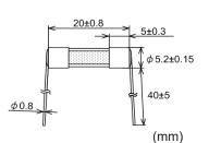
Tube:Lead-free glassEnd-cap:Nickel plated brassLead wire:Tin plated copperSolder:Pb90-Sn\*1Adhesive:Epoxy resinArc extinguishing material:ConfidentialMarking:SOC SHV11<br/>AC/DC400V [rated current]
