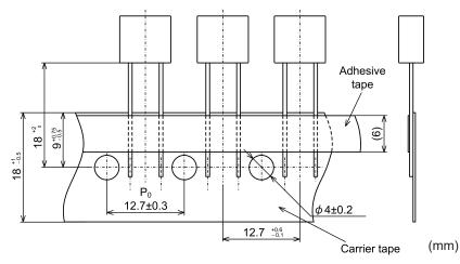
Specifications other than stated above shall be in accordance with JIS C 0806-2. Cumulative tolerance of the tape feed hole pitch ( $P_0$ ) shall be ±1 mm for 20 pitches.
