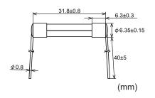
Tube: Lead-free glass End-cap: Nickel plated brass Lead wire: Tin plated copper
