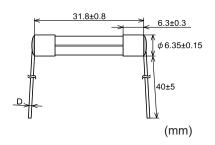
Rated current D Over 5 A-8 A:  $\phi \, 0.8$ Over 8 A-15 A:  $\phi 1.0$  Tube: Lead-free glass Nickel plated brass End-cap: Lead wire: Tin plated copper
