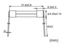
Rated current D Over 5 A–8 A:  $\phi$  0.8 Over 8 A–15 A:  $\phi$  1.0 Tube: Lead-free glass
