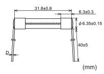
Rated current D  $100 \text{ mA-8 A:} \qquad \phi \ 0.8$ Over 8 A-15 A:  $\phi \ 1.0$ Over 15 A-30 A:  $\phi \ 1.2$  Tube: Lead-free glass
