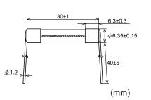
Lead-free glass End-cap: Nickel plated brass Lead wire: Tin plated copper Pb90-Sn\*1 Adhesive: Epoxy resin S < SOC [rated current] Marking: 250 V
